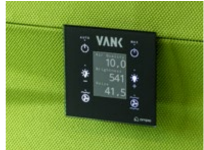
A 6-button wall-mounted touch pad with step lighting and ventilation adjustment and with air purity, lighting, and noise level sensors. Automatic or manual control.
